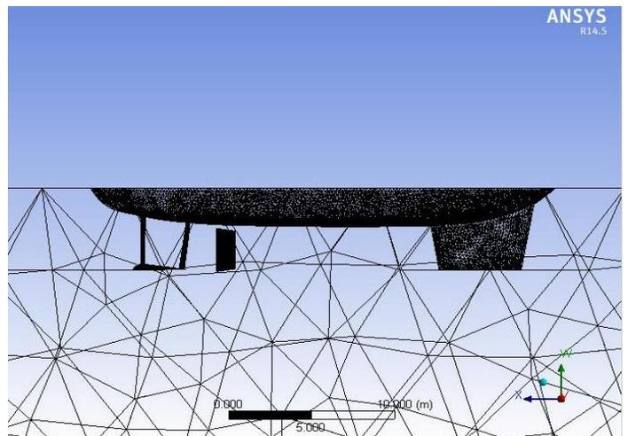
Figure 3. Mesh model of the static domain
