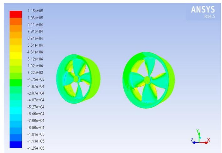
Figure 6. Pressure contour of the suction side (propellers and nozzle)
