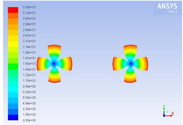
Figure 4. Velocity contours of the propellers
